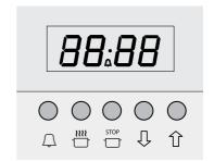
Figure 25 Clock display and control buttons
